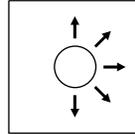
Air outlet angle 180° adjustable with adjusting wheels, e.g. in case of ceiling installation near walls
