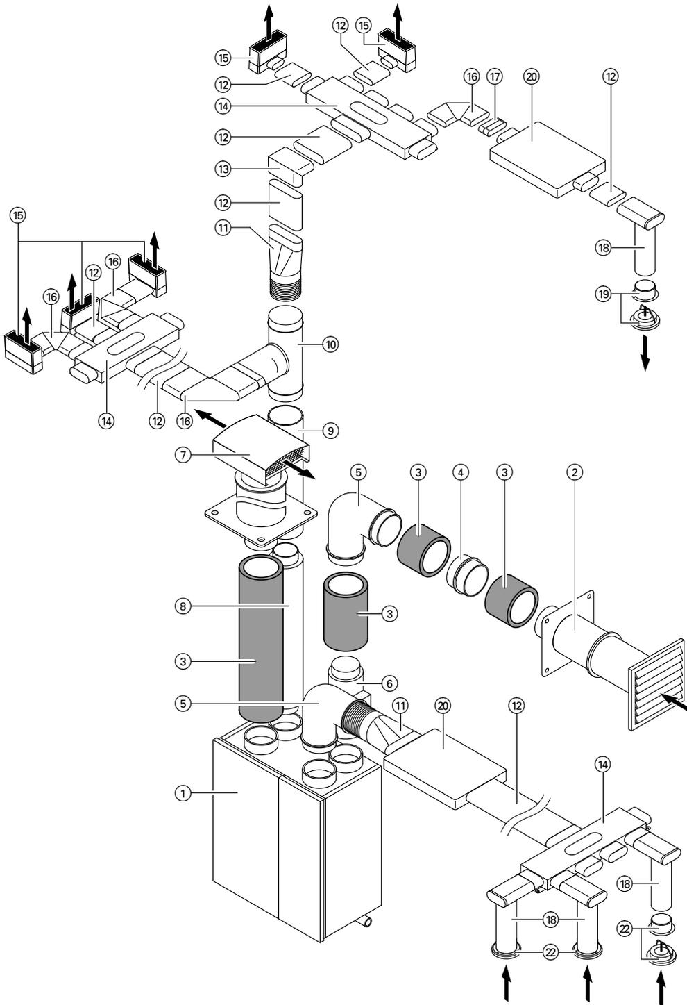
System illustration, metal duct system
