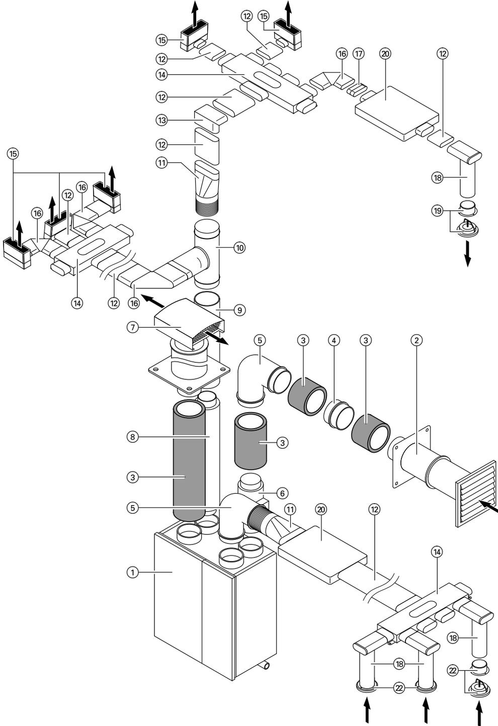
System illustration, metal duct system
