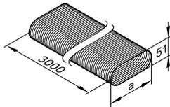
Made from zinc-plated sheet steel, ribbed inside.
