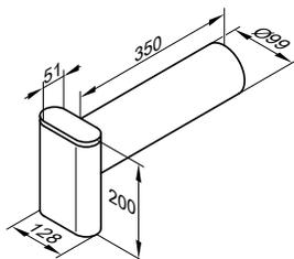
Adaptor from round duct system (DN 100) to flat (system 100)
