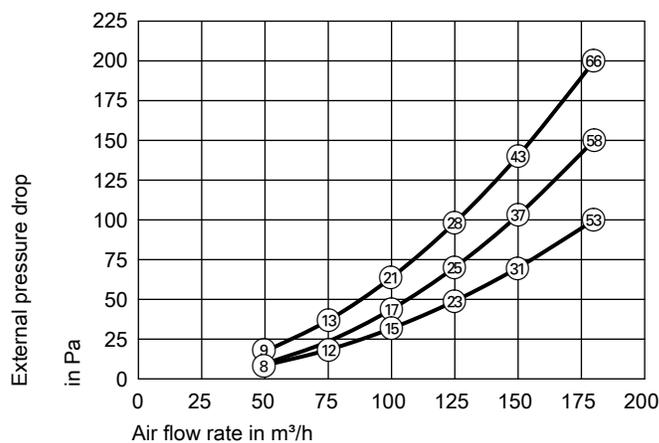
(x) Power consumption per fan in W at min. average or max. pressure drop
