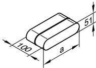
For joining flat duct elements (rigid or flexible).
