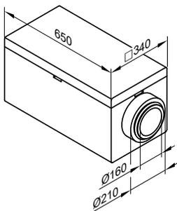
The internal ventilation air filter of the Vitovent can be removed if an outside air filter box is used.
