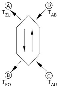
The outside air is preheated by the heat recovered from the extract air. In standard mode, the temperature-related heat recovery level  $\eta_{WRG}$  of the Vitovent 300 is in excess of 91 % (according to tests carried out by TZWL Dortmund [Germany]).
