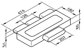
For the connection of 3 flat ducts, system 100
