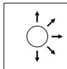
Air outlet angle 180° with fascia, e.g. in case of ceiling installation near walls
