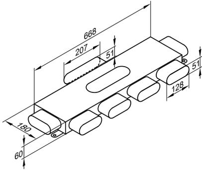
For the connection of 4 flat ducts, system 100
